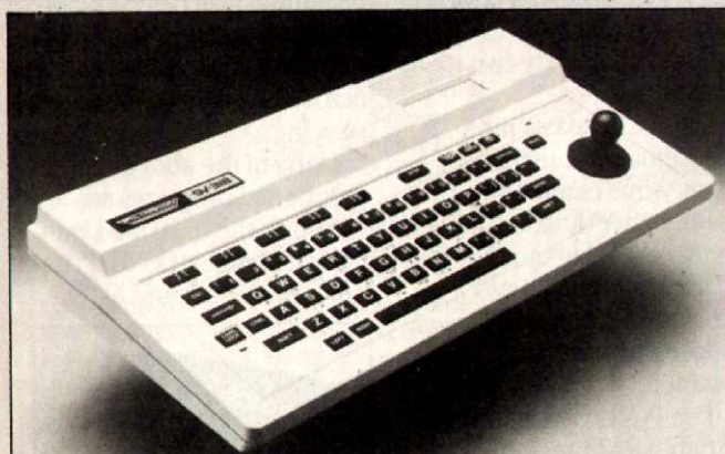
Pictured above is Spectravideo's SV-318 computer and the SV-601 Super Expander. With the addition of the Expander, the SV-318 system can interface with as many as seven additional input-output devices simultaneously. Special slots on the Expander, which face the user, monitor the operation of the interface cards connected to the system. Spectravideo is preparing fourteen hardware accessories for the system.
