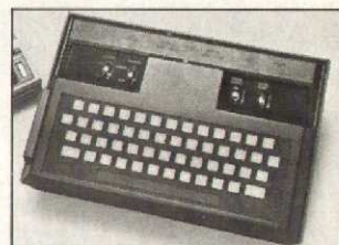
Atari's My Own Computer attaches to the cartridge slot and contains its own slot for peripherals.
