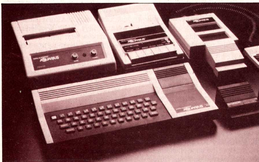
Mattel has ambitions of grabbing a portion of the home computer market. Shown here is their new Aquarius computer with its expandables: a printer, data recorder, computergame unit, and memory expanders.
