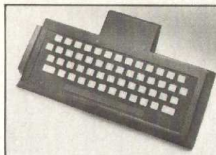
Atari's My Own Computer attaches to the cartridge slot and contains its own slot for peripherals.
