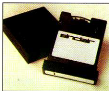
The mini 'disk drives' that Clive Sinclair promised on the original Spectrum adverts finally materialised in 1983. The Microdrives were actually tiny tape cartridges which could store and retrieve up to 100K of data at high speed. An add-on box followed which gave the Spectrum a cartridge slot and joystick ports. By this time, though, many games producers were using clever software methods to accelerate cassette loading so most Spectrum owners didn't see the need for the Microdrive, or a cartridge slot. And most already had a joystick adapter.
