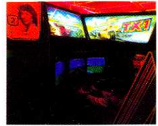
Atari's TX-1 was a driving coin-op that used three monitors placed side-by-side to give players a panoramic view of the action.
